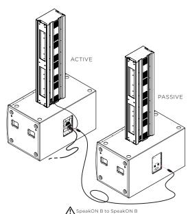
Once assembled, use the the 2m Cleaning Once assembled, use the 2 m (6.5 ft) long with a pair of cables connected to the XLR (6.5 ft) long speaker cable to connect one speakON connector on the GH412 rear the housing. Do not use any solvents, connector on the GH12 rear panel to on the GP18A active loudspeaker rear panel, panel to the speakON A connector on the chemicals, or cleaning solutions containing
