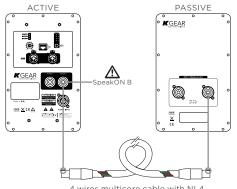
4 wires multicore cable with NL4 SpeakOn adapters
